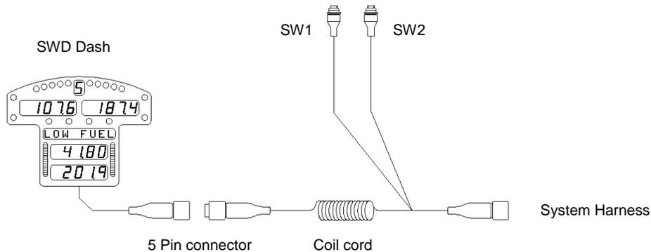
**Figure 15** - Typical SWD installation
