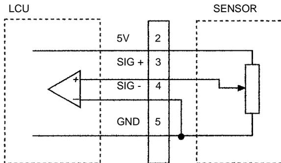
**Figure 22** - Connecting a single ended input
