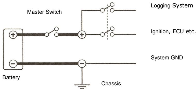
**Figure 6** - Battery Connections
