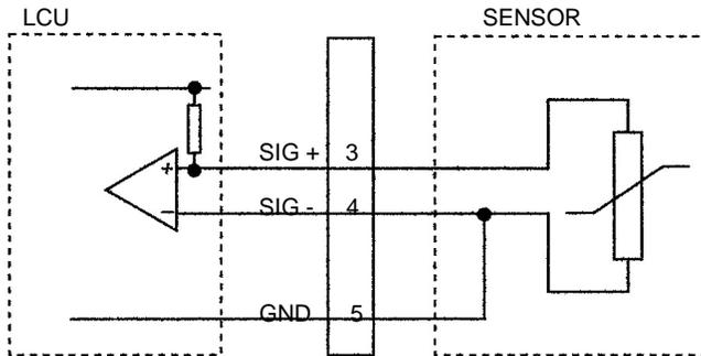
**Figure 24** - Connecting an RTD sensor
