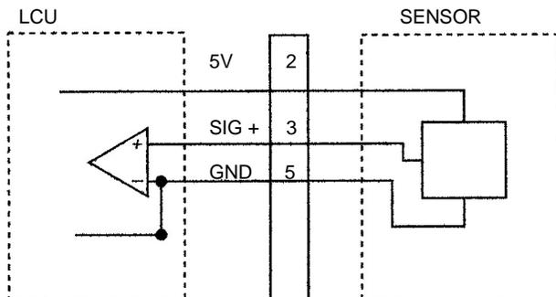
**Figure 25** - Connecting a voltage output
