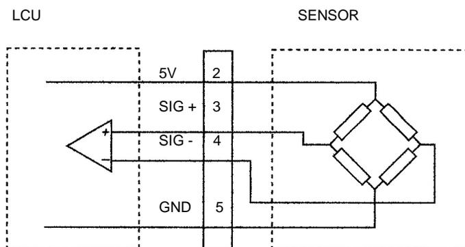
**Figure 23** - Connecting a differential input
