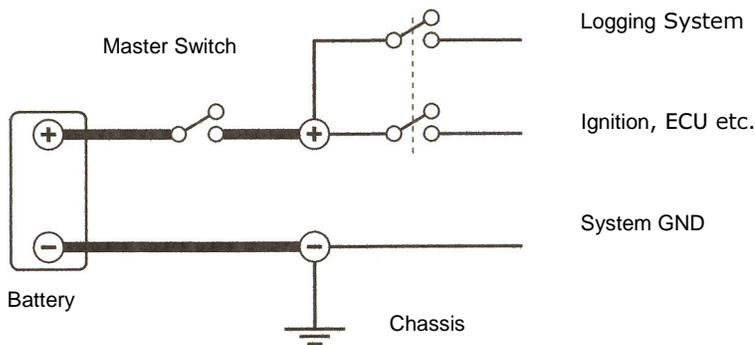
**Figure 6** - Battery Connections
