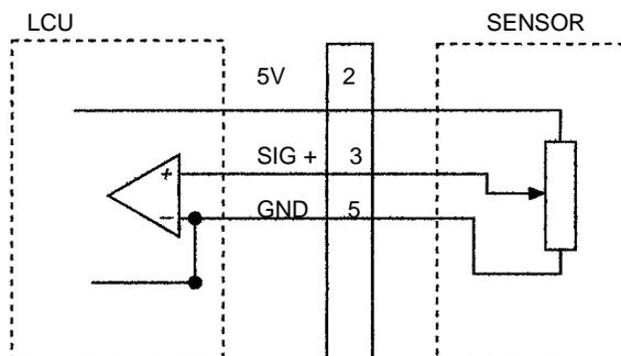
**Figure 21** - Connecting a single ended input
