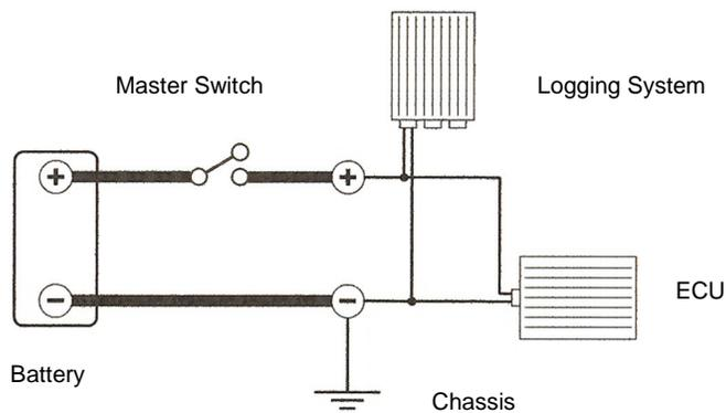
**Figure 7** - ECU Connections
